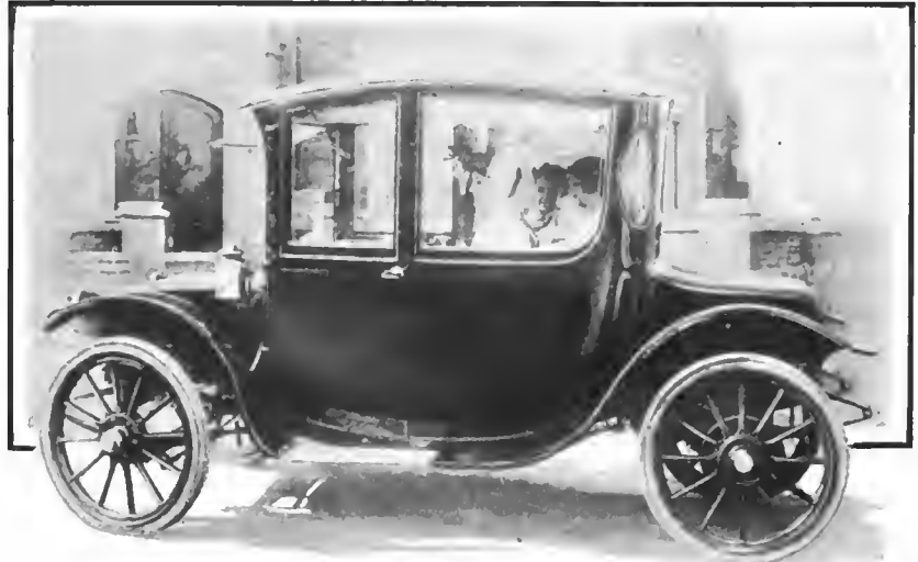
New Waverley four-chair Brougham, model 109. Note the rounded corners at the rear and the new shape of battery boxes at front and rear. The windows are larger and sashless
